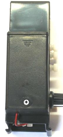
5) Reattach QuikFinder to baseplate, remove Phillips screw from battery holder to remove battery holder cover plate and insert 2 AA batteries and you're ready to go!
