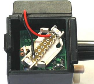
4) Tuck wires into notch and stick battery holder to side of QuikFinder using provided double sided tape.
