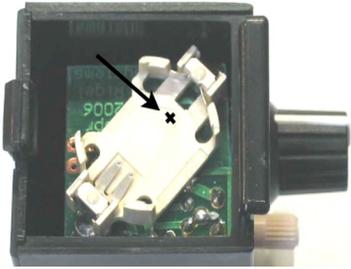
2) Place Quikfinder with knobs to right, side up as shown. 3/8<sup>th</sup> inch from back, make 1/4<sup>th</sup> inch deep notch in side using drill, clipper or other tool as shown. This will not void your warranty.
